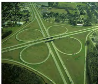
Motorists traveling along this clover-leaf interchange experience a normal acceleration due to the change in direction of their velocity. A tangential component of acceleration occurs when the cars' speed is increased or decreased.
